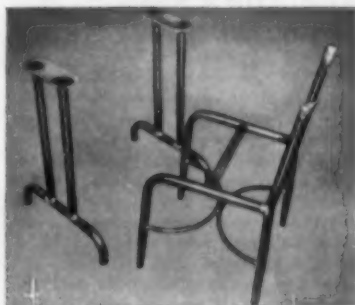
Braze welded frames for Peabody school furniture—combination of chair and open-front table.
